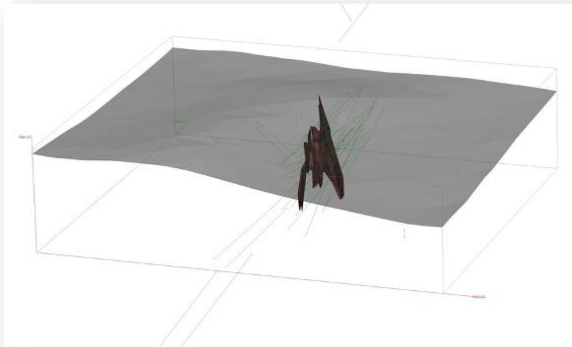
**Figure 14.5 Isometric view looking NNW of the Norra VMS Zone with surface topography and drillhole traces**
