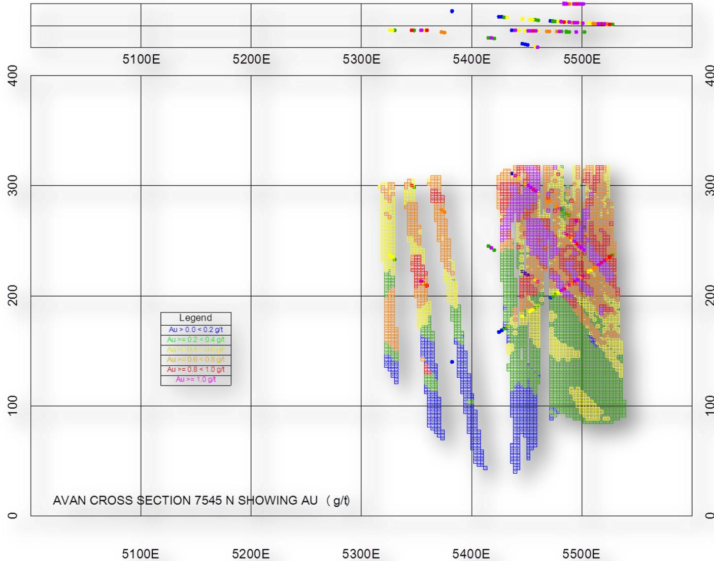
Figure 14.7 Avan Cross Section 7545 N Showing Au in Blocks and Composites
