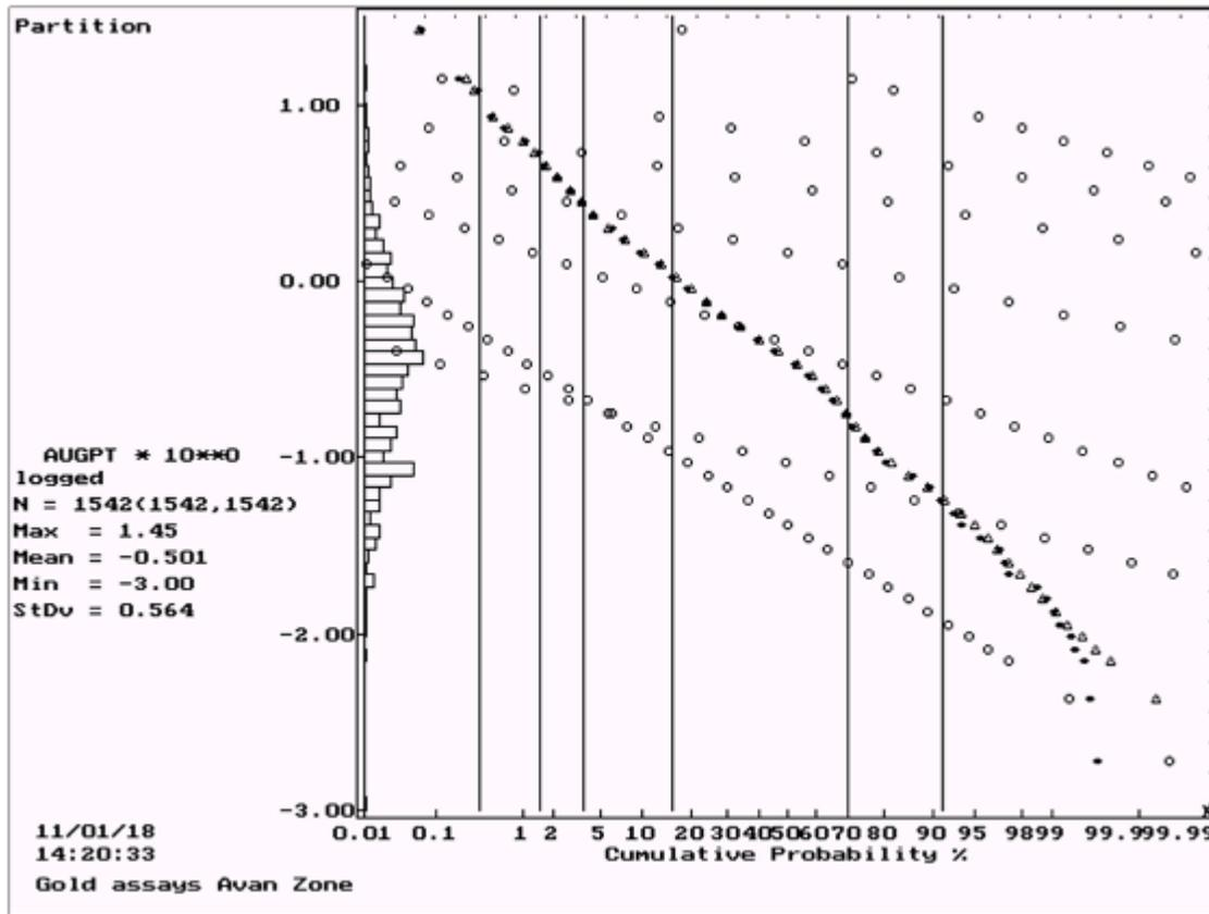
**Figure 14.3 Lognormal cumulative frequency plot for Au in the Avan Mineralized Zone**
