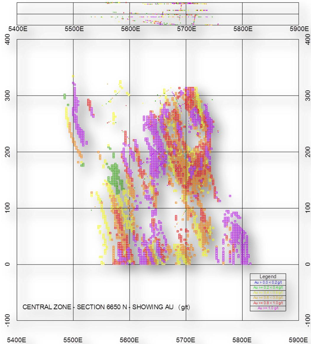
**Figure 14.8 Central Zone Cross Section 6650 N Showing Au in Blocks and Composites**
