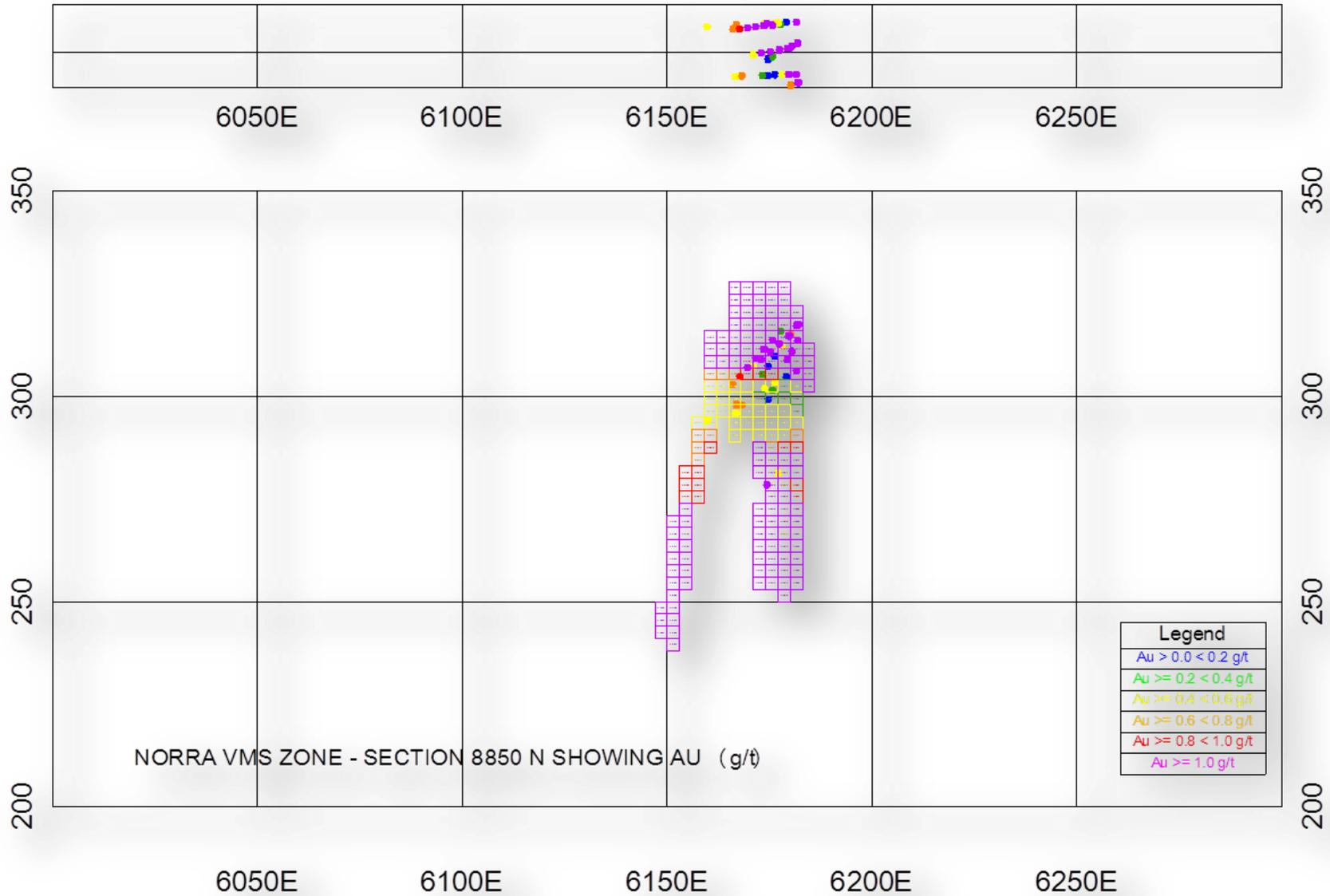
Figure 14.12 Norra Cross Section 8850 N Showing Au in Blocks and Composites
