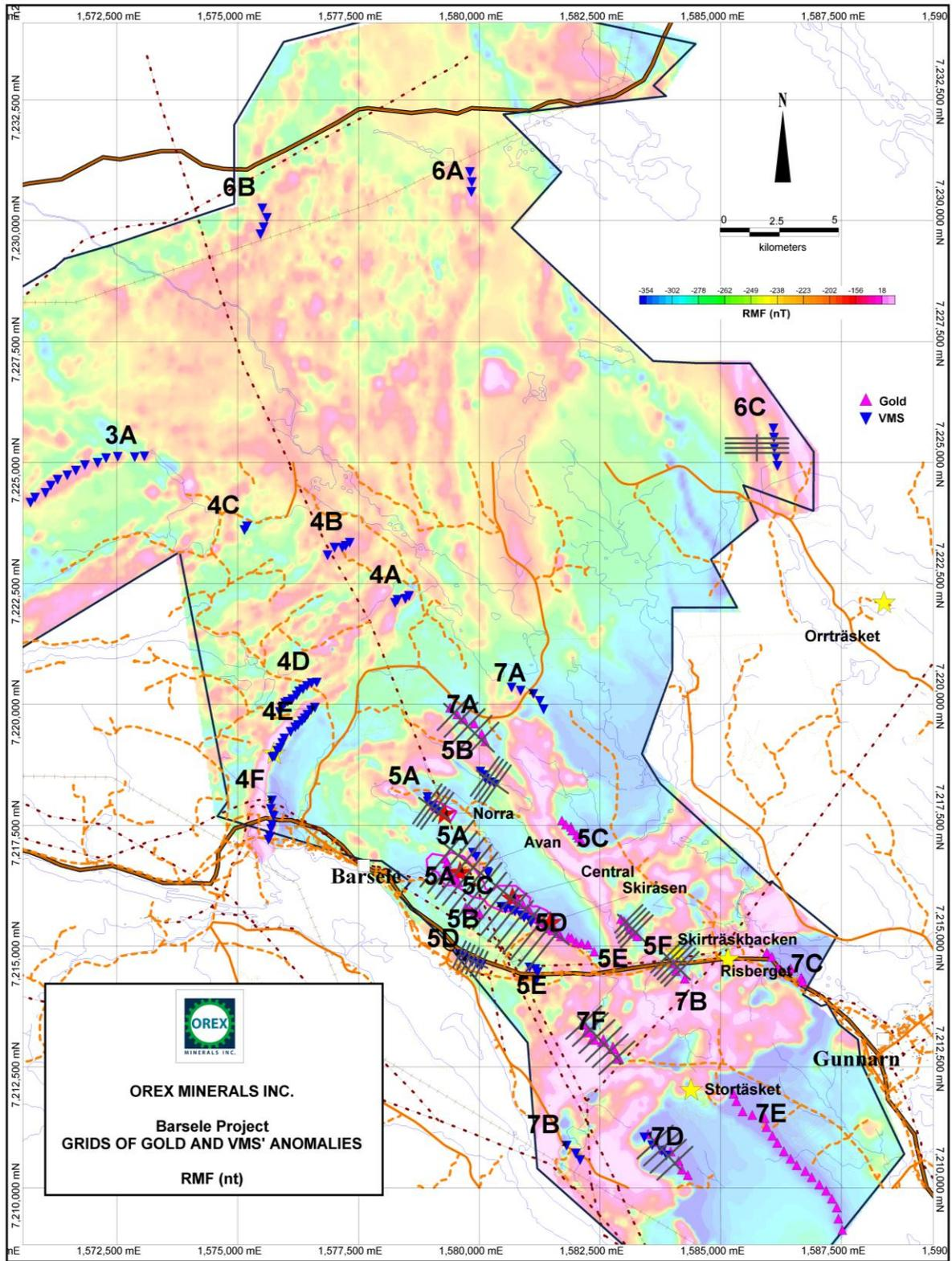
**Figure 9.2 Residual Magnetic Field (nT) of Airborne Survey Barsele 2011 with interpreted gold and VMS targets included as triangles and IP grid locations (Map Credit Orex, 2012)**
