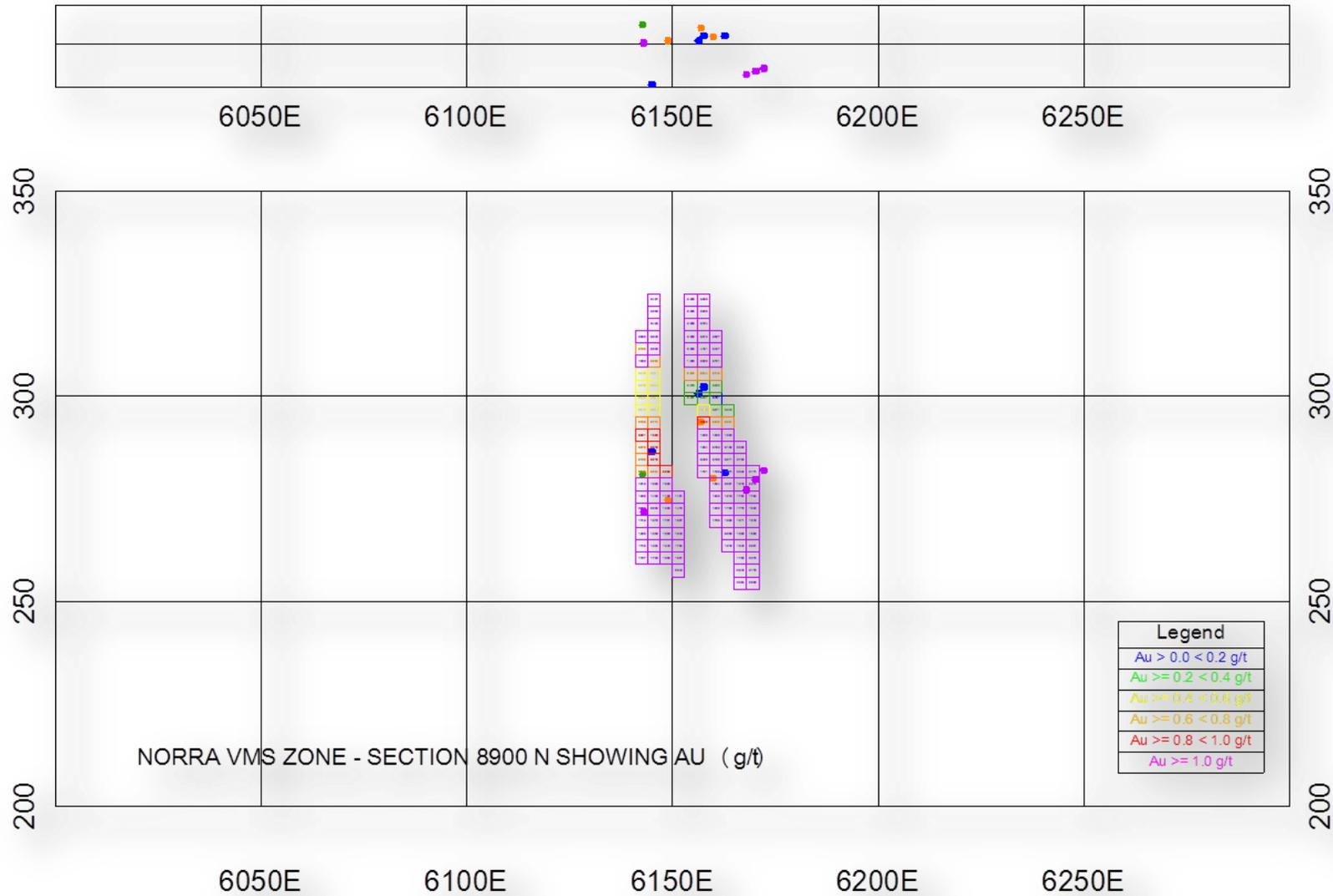
Figure 14.11 Norra Cross Section 8900 N Showing Au in Blocks and Composites
