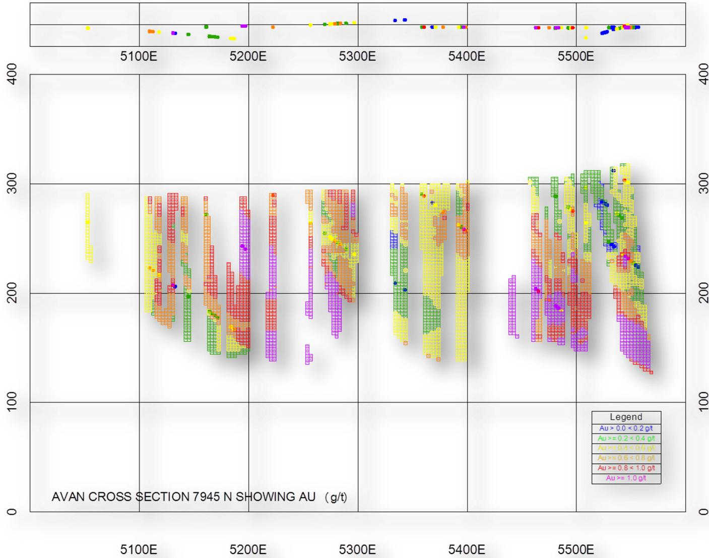
Figure 14.6 Avan Cross Section 7945 N Showing Au in Blocks and Composites
