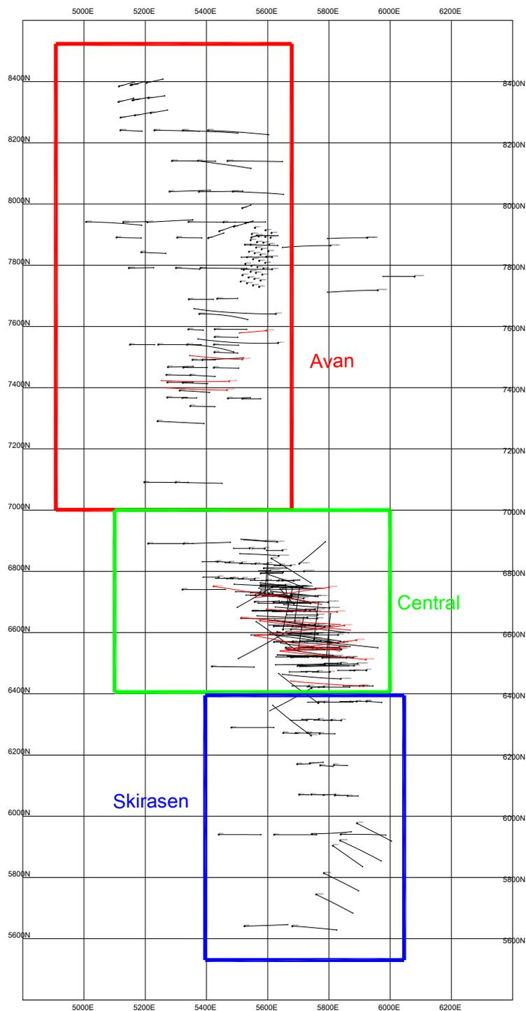
**Figure 14.1 2011-12 Drilling Relative to the Barsele Mineralized Zones. New drillholes shown in red in the Central and Avan Zones.**
