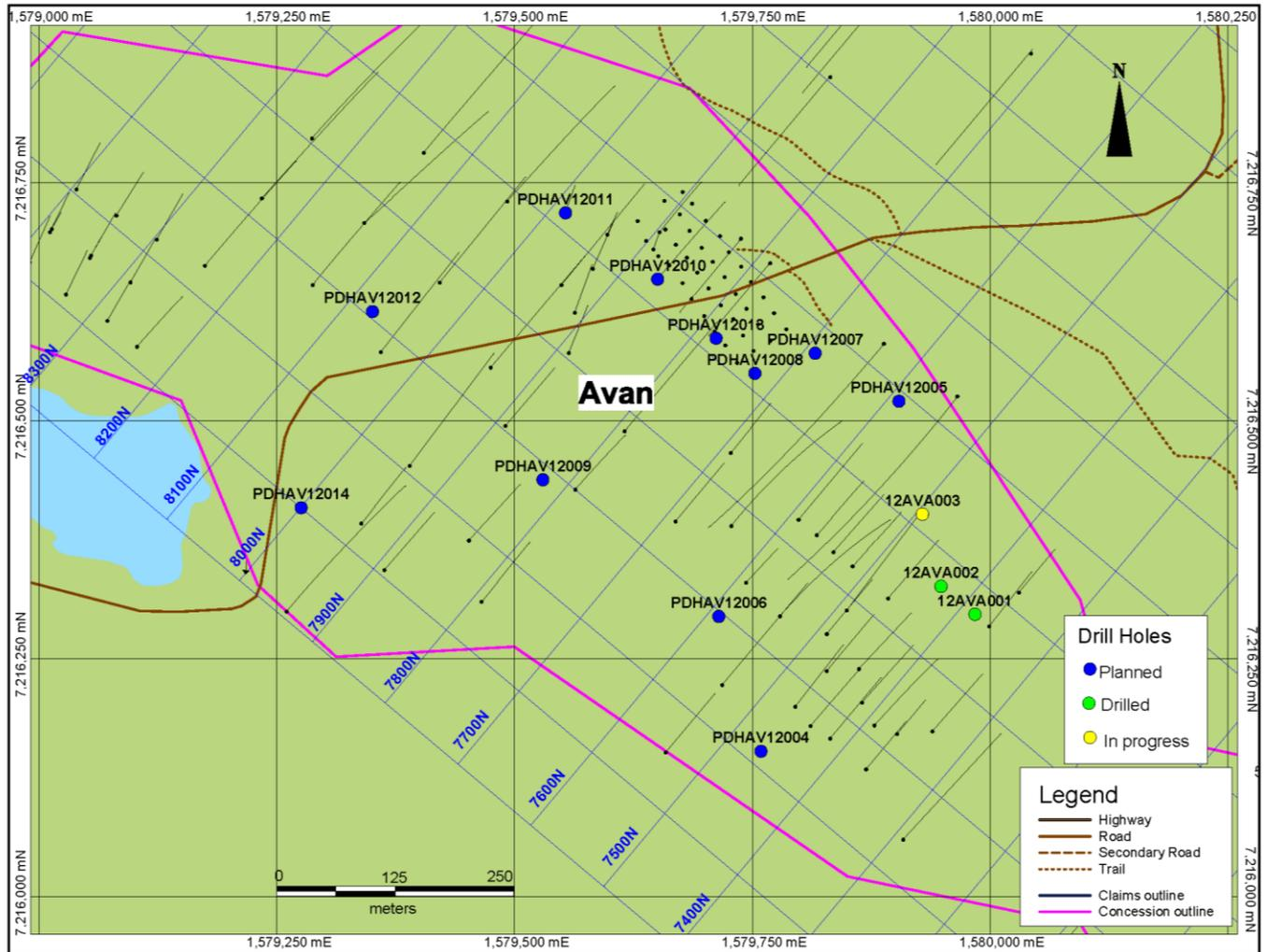
Figure 10.5 Plan View of Drilling Collars – Avan Zone (Map Credit Orex, 2012)
