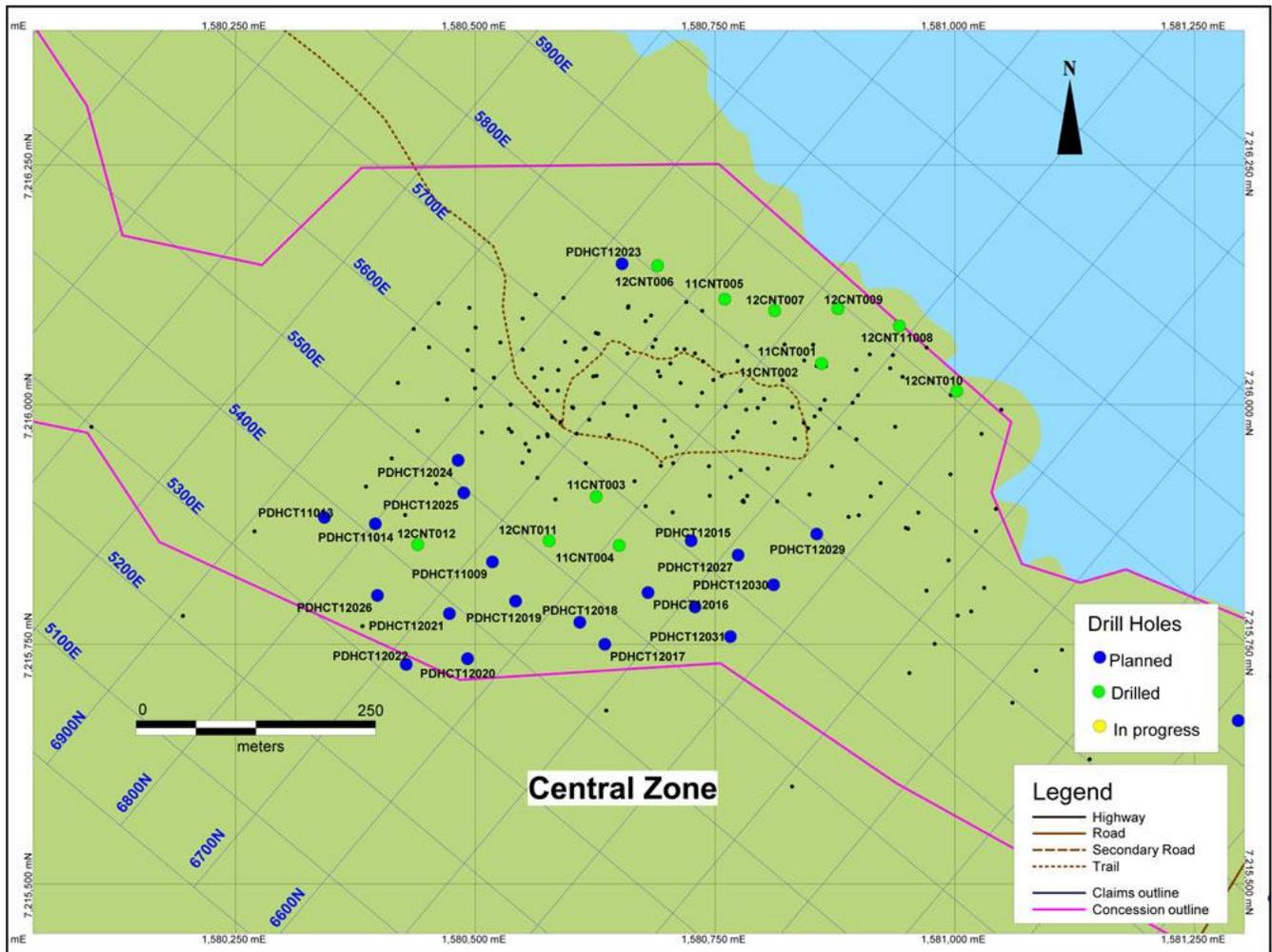
Figure 10.1 Plan View of Drill Collars – Central Zone (Map Credit Orex, 2012)
