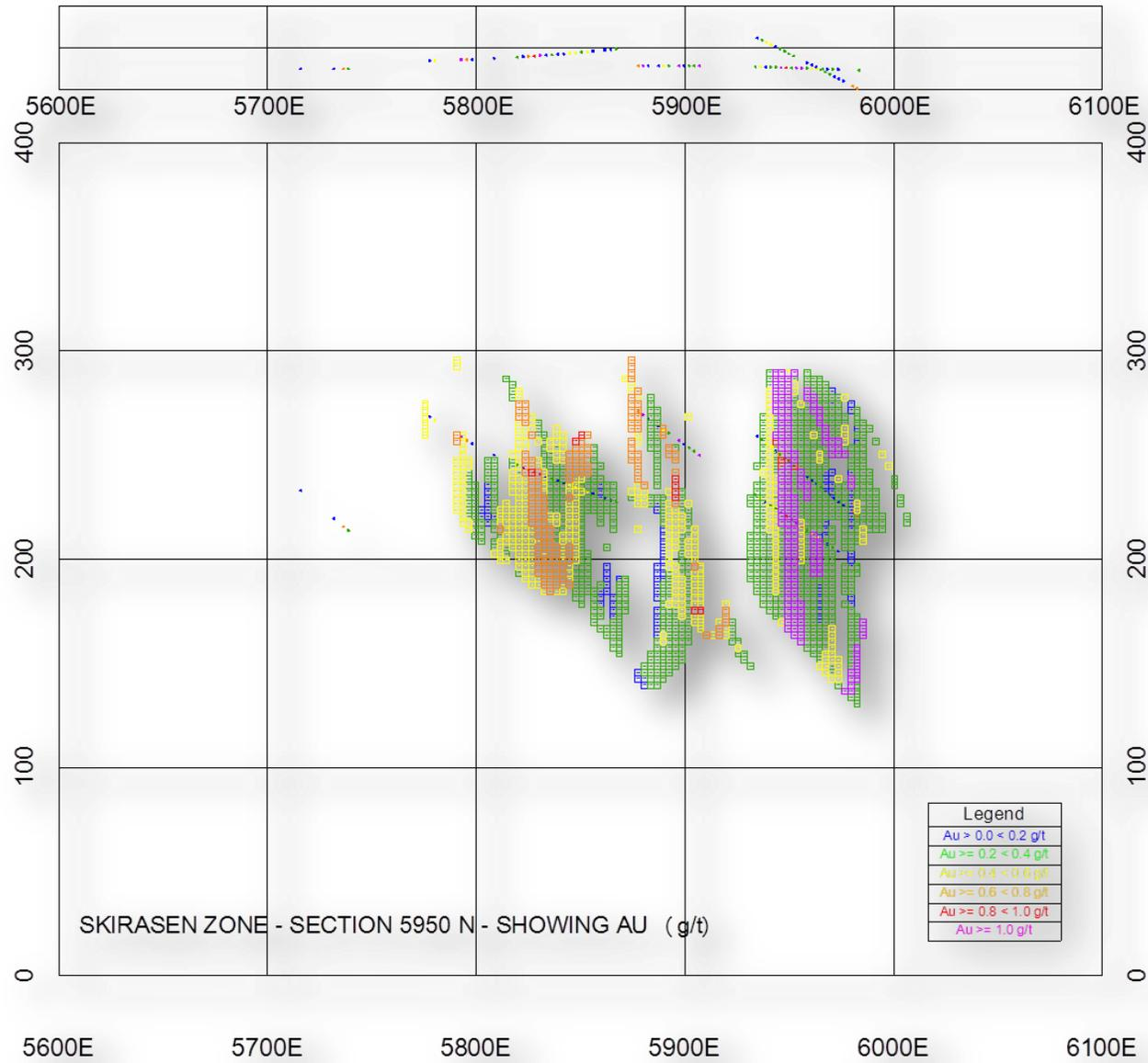
Figure 14.10 Skiråsen Cross Section 5950 N Showing Au in Blocks and Composites
