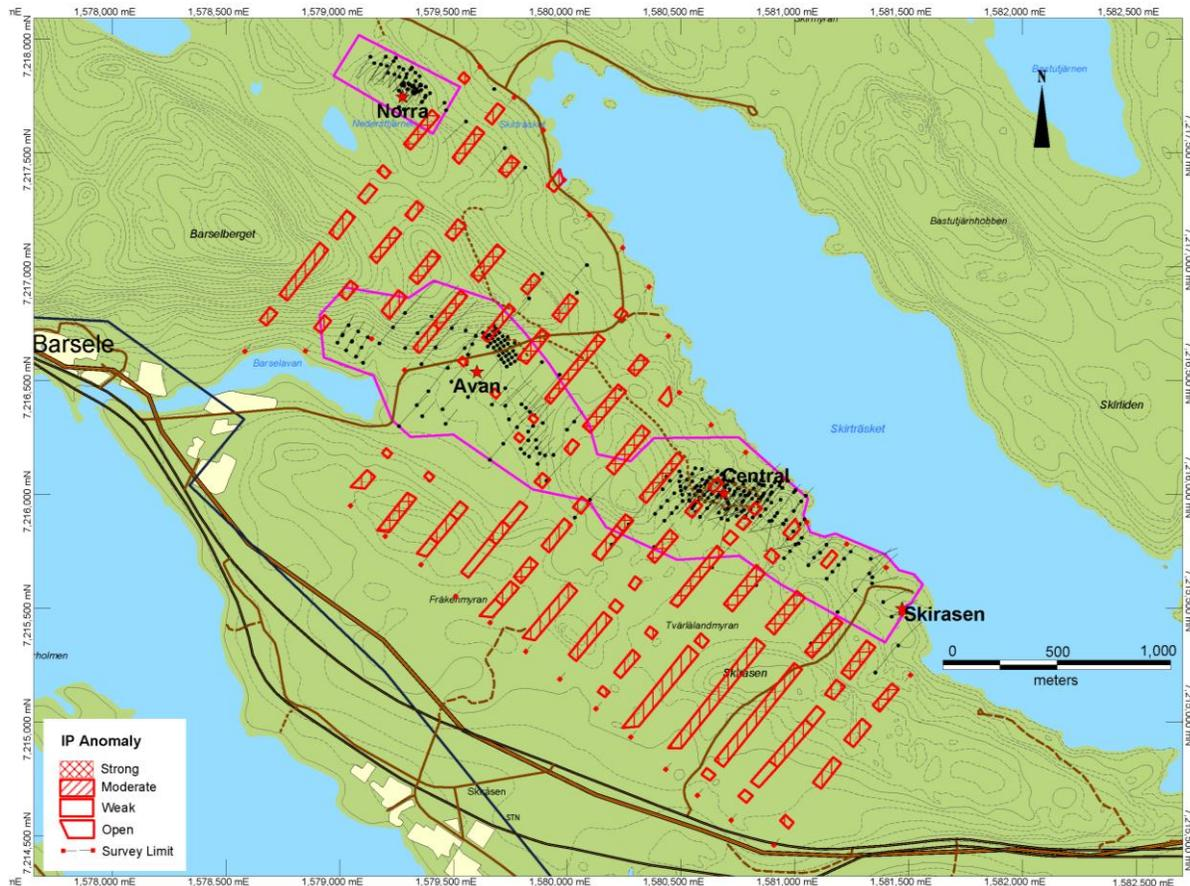
**Figure 9.3 2011 Induced Polarization Survey plan over Central and Avan zones (Map Credit Orex, 2012)**
