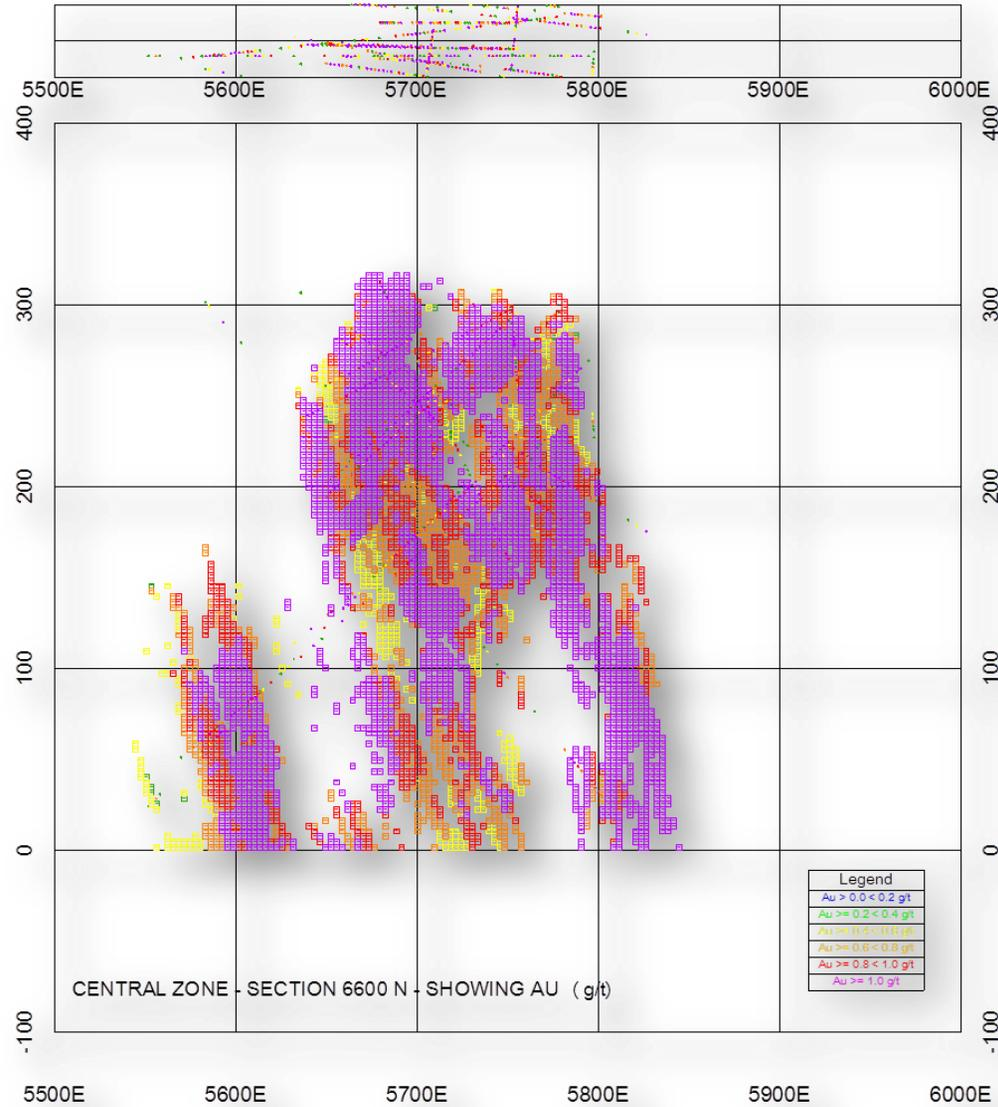
**Figure 14.9 Central Zone Cross Section 6600 N Showing Au in Blocks and Composites**
