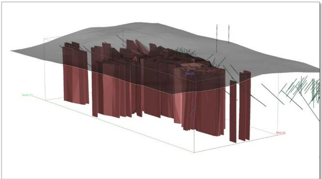
**Figure 14.2 Isometric view looking NE showing Avan Solid, surface topography and drillhole traces**
